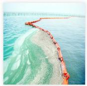
It is a kind of economical and universal oil containment boom, especially suitable for intercepting and controlling oil spills and other floating objects in coastal calm waters. It can be fixed for a long time. It has been widely used in inland pollutant discharge entrance, river, harbor, lake, offshore oil drilling platform and other waters..
